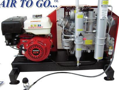
Charging rate 6.6 SCFM\*\*; 5.5 F.A.D. (Fill time for 80 cu. ft. cyl 12 min\*) Will fill SCBA's to 4500 psi Breathing air quality meets or exceeds: NFPA 1500 CGA "E" EN 12021 ISO 9001: 2008
