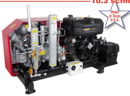
Charging rate 10.8 SCFM\*\*; 9.0 F.A.D. (Fill time for 80 cu. ft. cyl 7.5 min\*) Will fill SCBA's to 4500 psi
