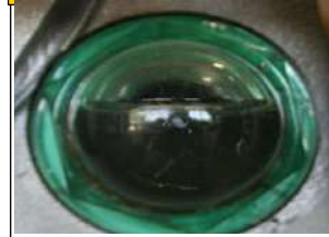
Figure 1. Oil Level Sight Glass
