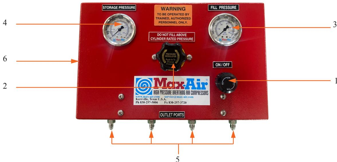
1. On/Off Valve – clockwise to close, counterclockwise to open
